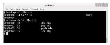
figure 67 - Disassembly of default module\_mz\_x86 value
